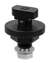
The Uni-Bolt fastens fixtures or pipes to strut channel. Insert the Uni-Bolt into the strut channel, rotate 90 degrees and spin the 2" diameter knurled disk to lock into the channel. Also available for 1 5/8" x 13/16" strut channel.
