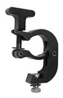
The TC Clamp will fasten from 2" OD to 1.5" OD tube. The TC Clamp has a 2-1/2" T-handle so no tools are required to fasten to the pipe. 1.25" x 1/2"-13 TPI Grade 8 fastener, Nylock Nut and 1" diameter Belleville Spring washer are provided for connecting your load. Dimensions: 4-5/8" Tx 4"W x 1-3/16" thick. Safe Vertical Working Load 450 Pounds, (200 KG). Weight is 1.22 pounds (.55 KG)
