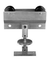
The Scenery Carrier is adjustable to fine tune the height or leveling of your flats or other scenery elements. Turnbuckle style bolt makes for quick adjustments by turning the knurled disk. Two holes are provided for #10 wood screws.
