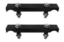
Made in the USA, the Mega-Grapple is made from billet aircraft 6061-T6 aluminum. It is perfect for creating "T" sections of box truss. Sold in pairs with two 5/8" x 4" bolts, washers, nuts. Includes spacers to protect the truss.
