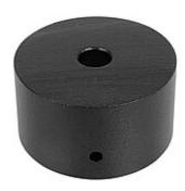
The Mega-Coupler Pipe Adapter Flush can be used to rig pipe-mounted plasma screens, projectors and speakers from overhead pipe or truss. The Mega-Coupler Pipe Adapter Flush connects onto an 1-1/2" NPT threaded pipe on one end and uses a 1/2" bolt to connect onto the desired mounting surface. The Mega-Coupler Pipe Adapter Flush has a 1/4-20 set screw to secure the pipe threads and an inspection hole to verify that the pipe is fully inserted.
