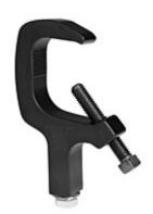
The world's standard theatrical lighting c clamp, the Mega-Clamp, is created from high tensile, aircraft grade, extruded aluminum. The Mega-Clamp's 600 pound design load is twice as strong as most cast iron
